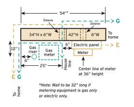
Note: Block wall specifications must meet all municipal codes. All voids in the blocks to be filled solid with concrete and contain minimum #3 rebar. Service sleeves for gas and electric house lines to be at 18 inches height.
