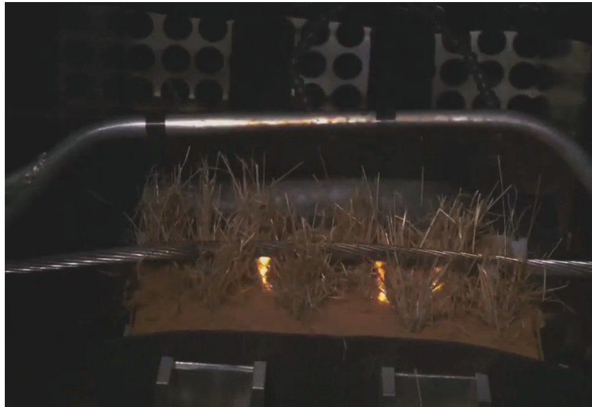
Figure 1-2. Test with REFCL Technology Enabled 2
